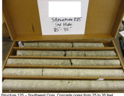
Structure 125 – Southwest Core. Concrete cores from 25 to 35 feet.
