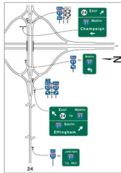
Fig. 2D-21. Example of Transposed Alignment Crossroad Guide Signing at Diamond Interchange from MUTCD
